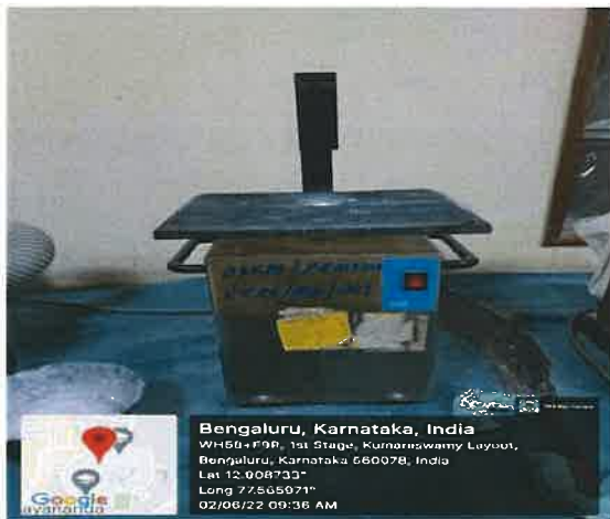
Pindex – to make pinholes in die or casts.
